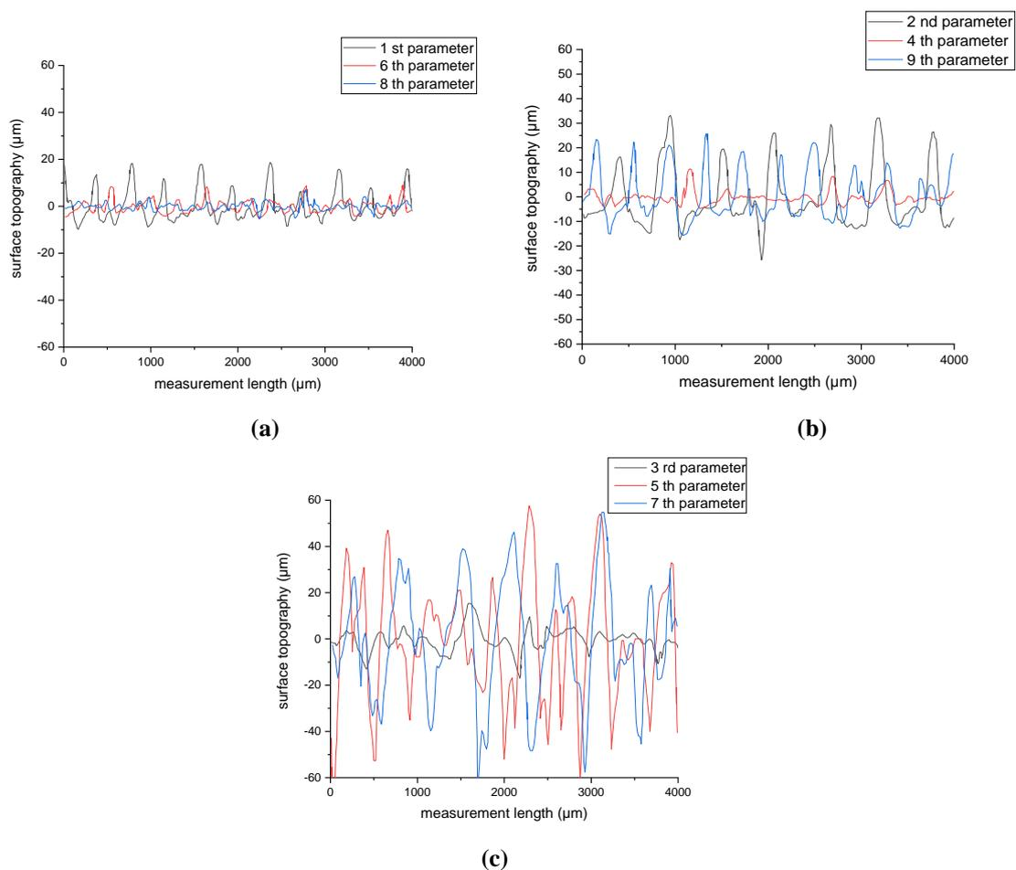
Fig. 3. Topographic graph with LH of (a) 0.1 mm; (b) 0.2 mm; (c) 0.3 mm.
