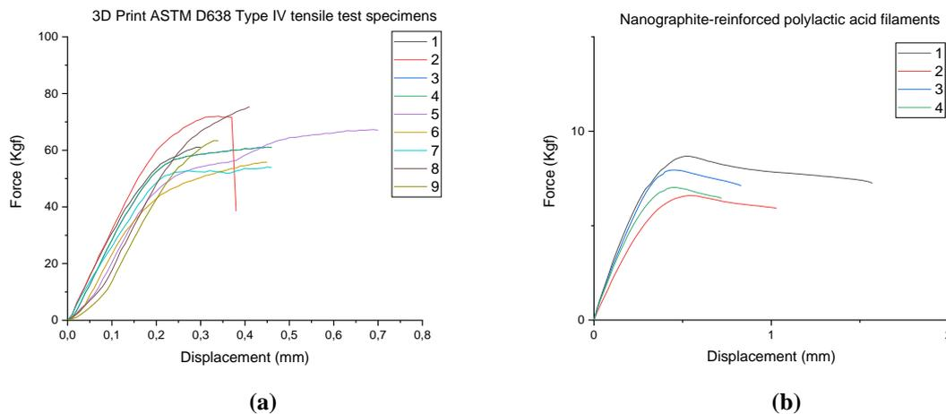
Fig. 4. (a) Force and displacement of the 3D-printed specimen; (b) Nanographite-reinforced PLA filament
