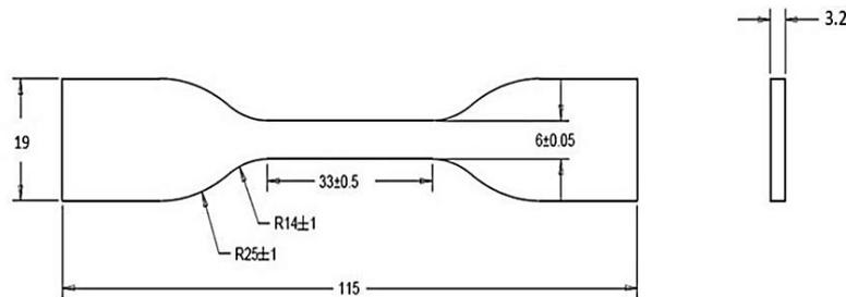
Fig. 2. Tensile test specimen ASTM D638 type IV
