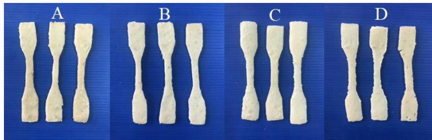
Fig. 1. Specimen \sigma_{UTS} ASTM D 638 type IV
