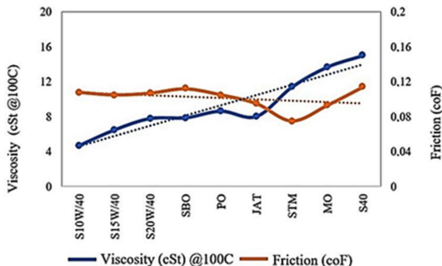
Fig. 2. Graph of Viscosity - Coefficient of friction [16-21]
