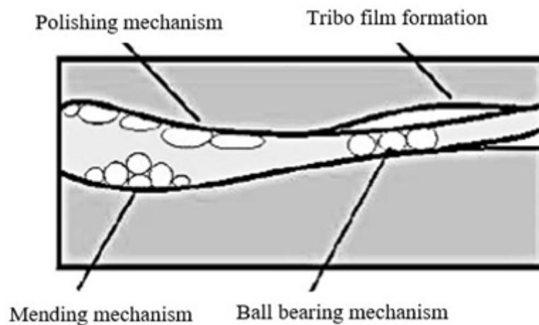
Fig. 1. Lubrication mechanism on two contact surfaces for lubricating nanoparticles [9].
