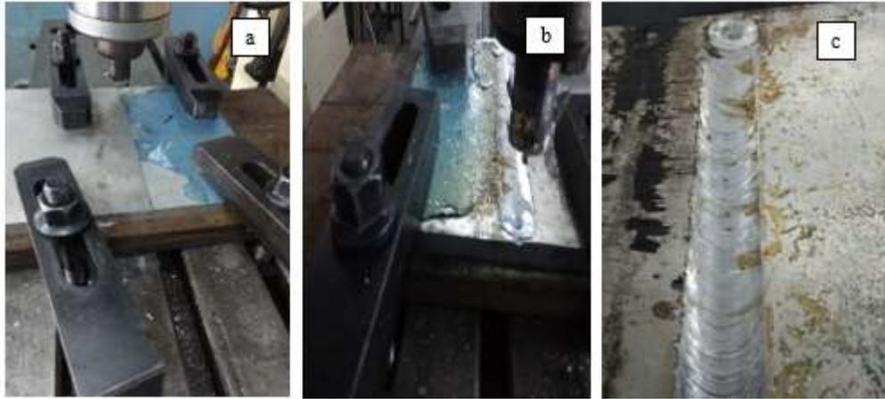
Fig. 7. a) FSW aluminum 6061 setting process, b) The FSW process is ongoing, c) Result of FSW the process in single U design
