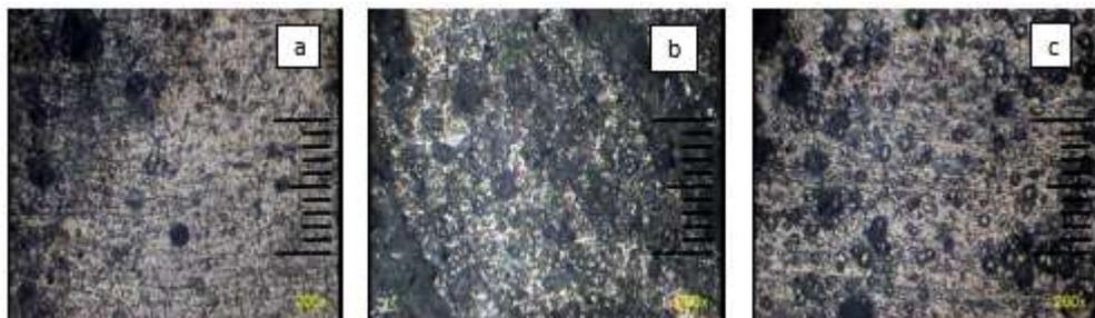
Fig. 11. (a) HAZ microstructure, (b) nuggets and (c) TMAZ double U joining 200 x magnification
