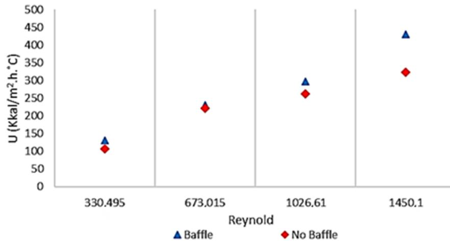
Fig. 7. Correlation graphs between overall heat transfer coefficient and the Reynolds number in two tests: with baffle and without baffle
