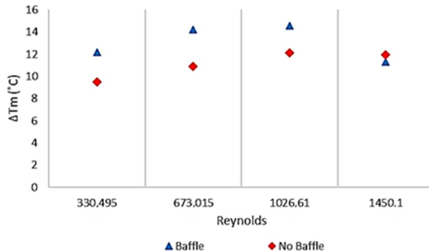
Fig. 4. Correlation graphs between the average temperature difference and the Reynolds number in two tests: with and without baffle
