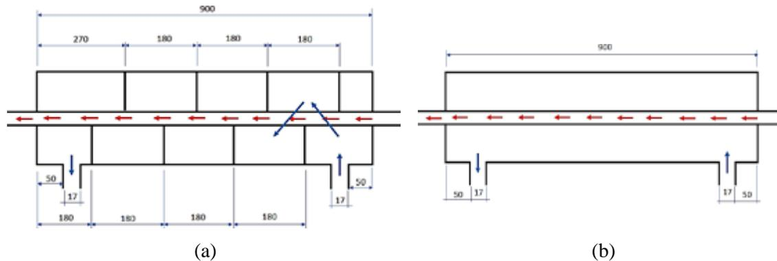
Fig. 3. Dimensions and water flow direction (a) Heat exchanger with baffle, (b) Heat exchanger pipe without baffle
