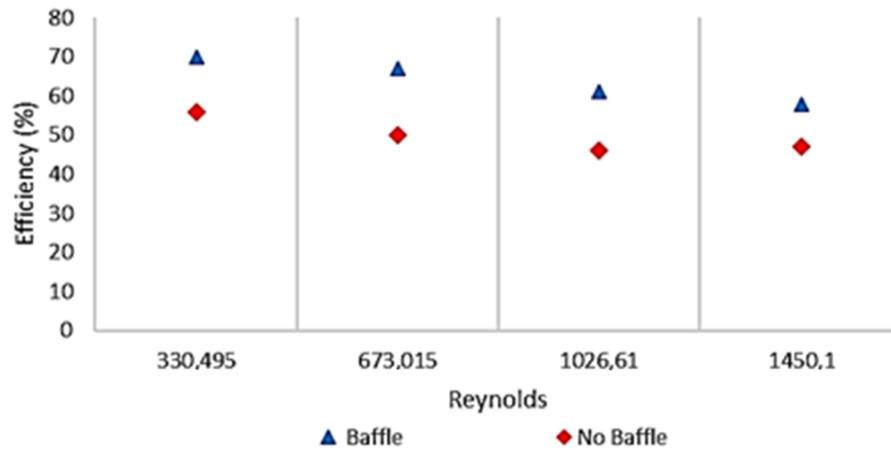
Fig. 6. Correlation graphs between heat exchanger efficiency and the Reynolds number in two tests: with baffle and without
