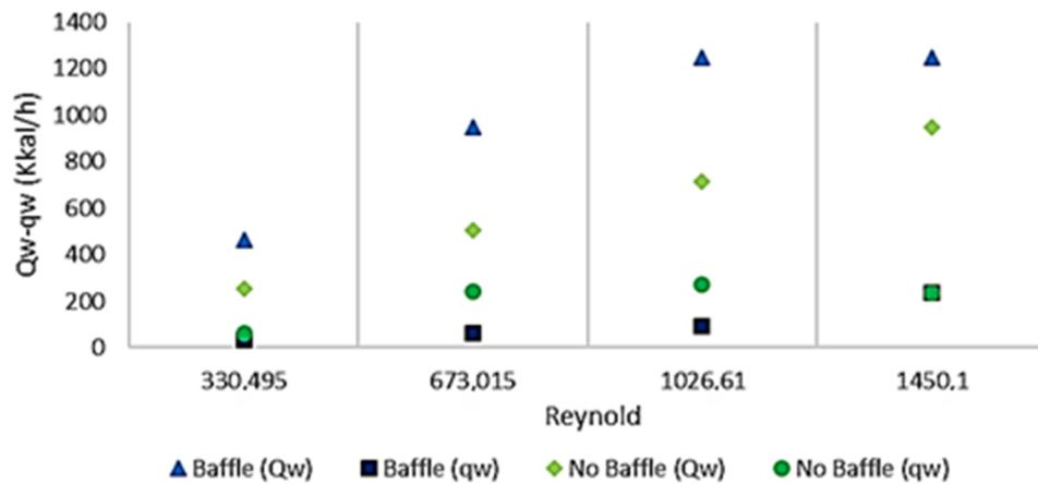
Fig. 5. Correlation Graphs Between Hot and Cold Water Heat Transfer and the Reynolds Number in Two Tests: baffle and no baffle
