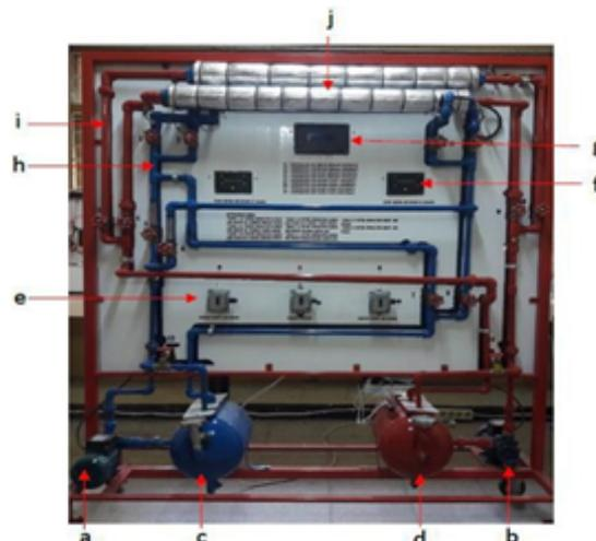
Fig. 2. Shell and tube heat exchanger (a) Cold water pump, (b) Hot water pump, (c) Cold water tank, (d) Hot water tank, (e) Switch, (f) Flow meter, (g) Thermometer digital, (h) Cold water line, (i) Hot water line, (j) Heat exchanger pipe baffle and no baffle
