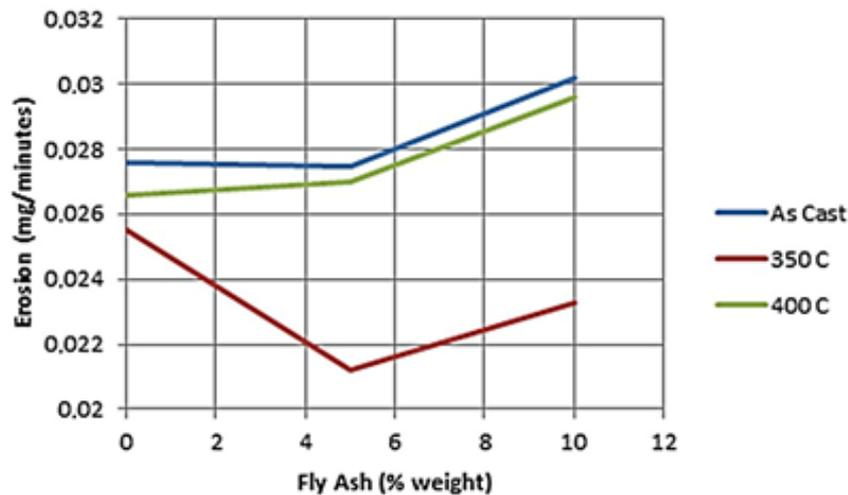
Fig. 3. Effect heat treatment to the erosion rate of brass composite
