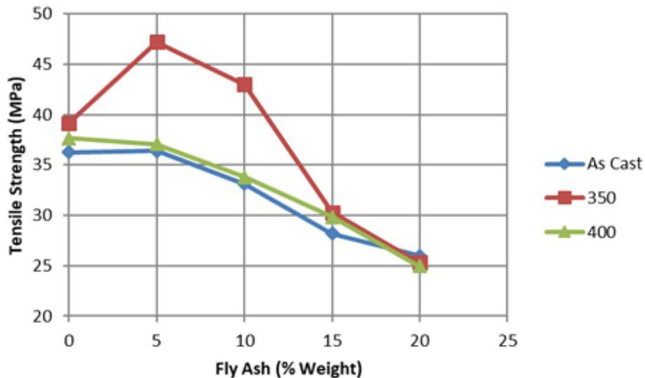
Fig. 2. Tensile strength of brass composite
