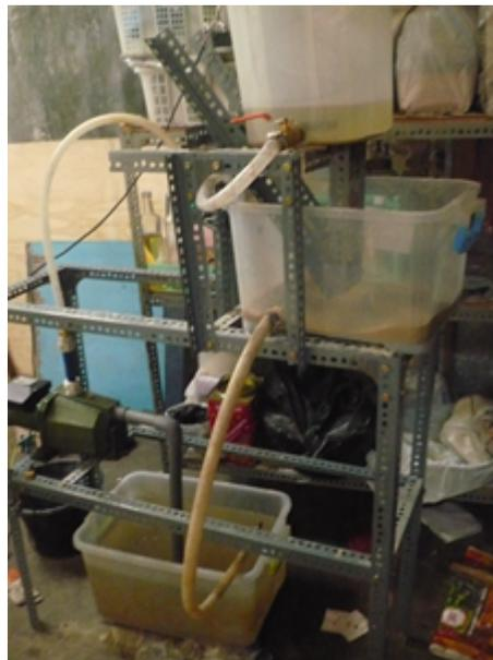
Fig. 1. Abrasive test apparatus
