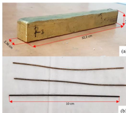
Fig. 1. Cu-21Zn-5Al alloys (a) as cast; (b) after the machining process
