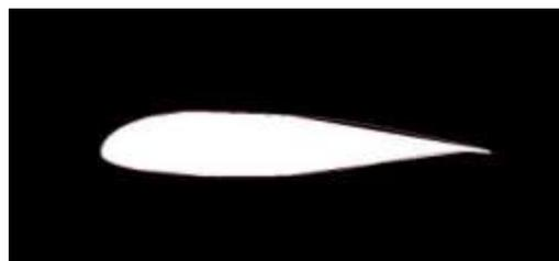
Fig. 1. The airfoil of LS (01)-0417 MOD [9]
