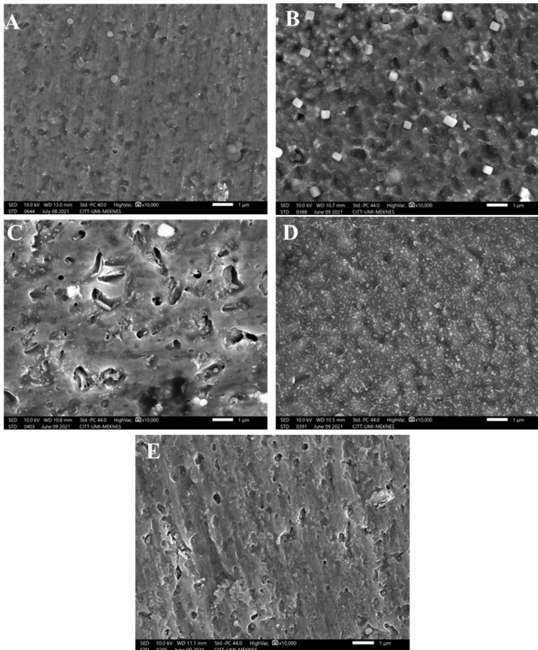
**Figure 3.** SEM photomicrograph of AA2024 T3 alloys: (A) control sample, (B) quenching sample, (C) homogenization sample, (D) artificial aging sample, and (E) recrystallization sample.
