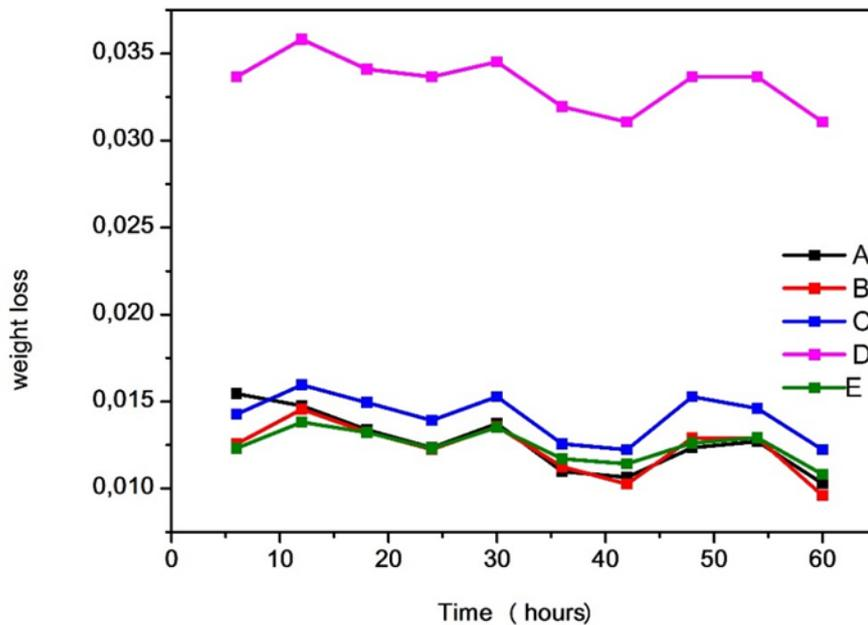
**Figure 5.** mass loss of the alloy as a function of immersion time in the AA2024 T3 climatic chamber (A) control sample, (B) quenching sample, (C) homogenization sample, (D) artificial aging sample, and (E) recrystallization sample.
