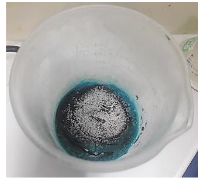
Fig. 4. The dried blue gel after removing all water components from the solution.
