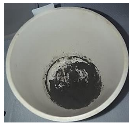
Fig. 7. The final product of \text{La}_2\text{CuO}_4 nanoparticles.
