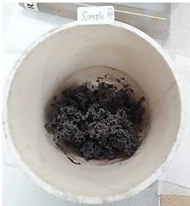
Fig. 5. The sponge-like product after the calcination process.
