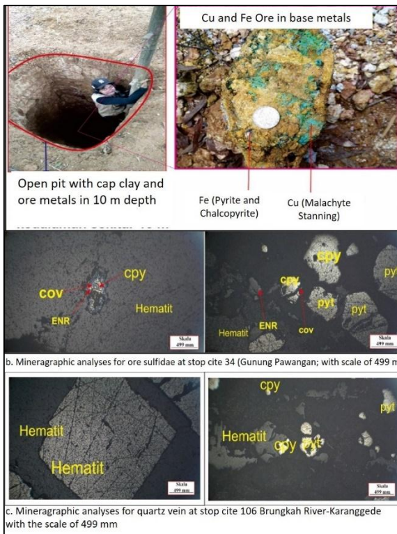
Fig. 8. Fe and Cu base metals in hand specimens (a), and the photomicrograph of polish incision for altered breccia (b) and quartz vein (c)
