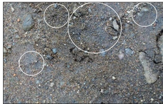
Fig. 11. Iron ore grains which spreaded in the alluvium deposits on the surface of the research area unevenly (source: personal documentation).
