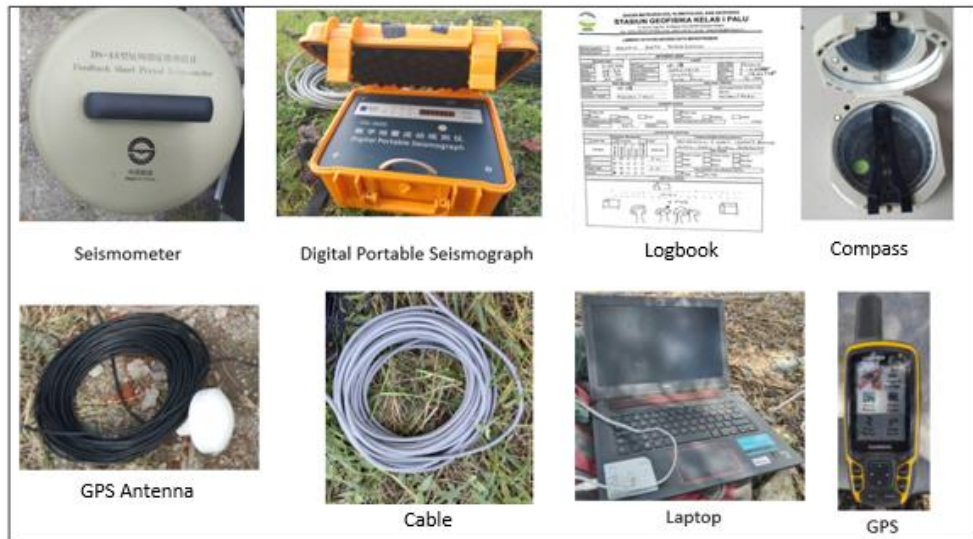
Fig 2. Microtremor data acquisition equipment
