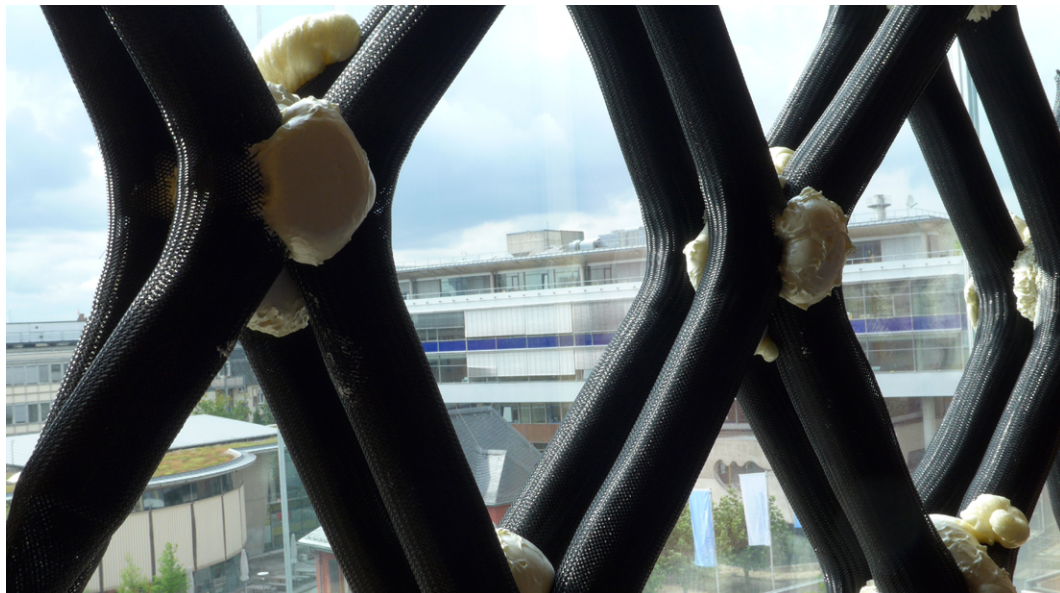
FIG. 7 Fully-fashioned, multi-layer structure consisting of pressure-resistant lightweight ropes made of foamed textile sleeves , © FFin.
