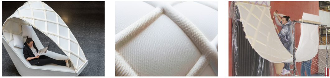
FIG. 4 Shell structure, made of fully-fashioned foamed spacer fabric, FFin © 4a+b Christoph Lison, ©4c FFin.
