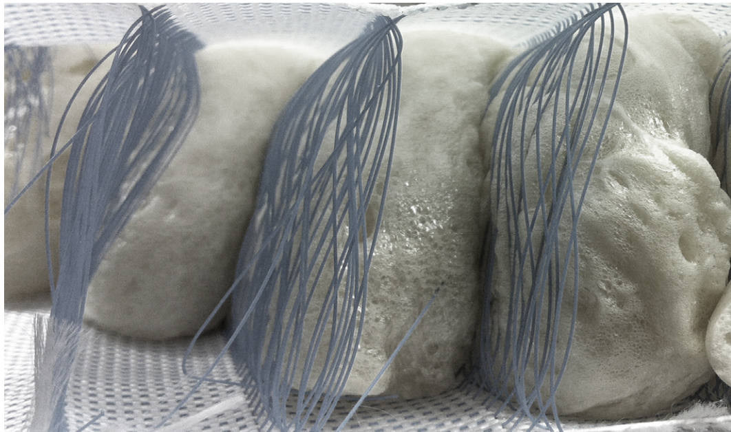
FIG. 1 3dTEX: Spacer fabric, filled with foam, FFin / ITV Denkendorf, ©FFin
