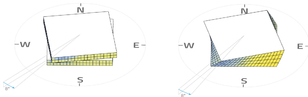
FIG. 5 Two façade types at 8^\circ floor-to-floor rotation angle
