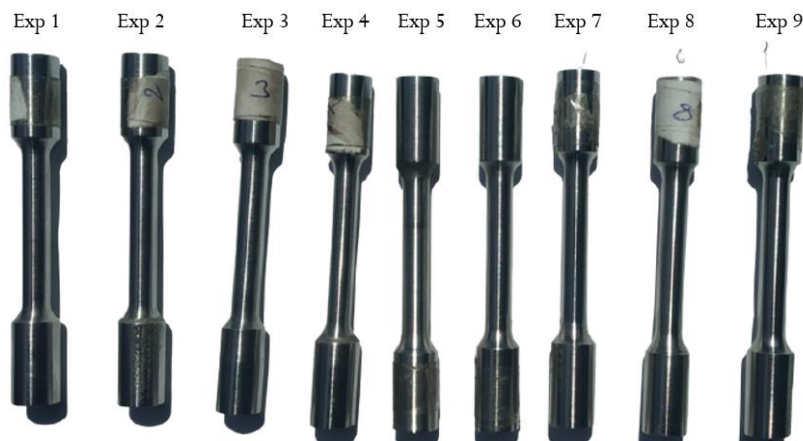
Figure 3. Tensile test specimens in L9 experimentation
