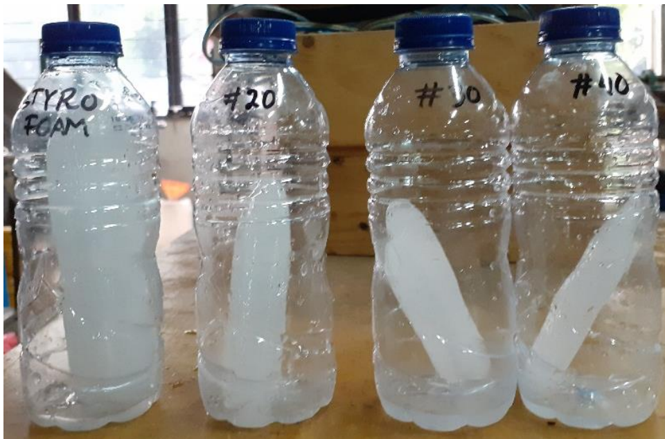
Figure 8. The condition of the ice cubes on some mesh coolboxes composite and box styrofoam after 4 hours
