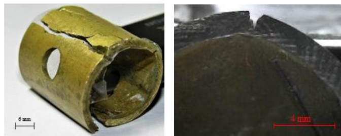
Figure 8. Specimens Condition After Immersion for Dezincified (left) and Non-Dezincified (right) Specimens
