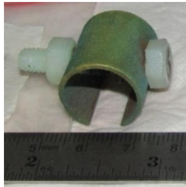
Figure 4. C-Ring Specimen following ASTM G38.
