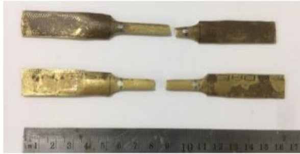
Figure 3. Tensile Test Specimen in Accordance with ASTM E8.
