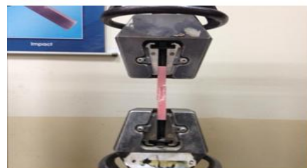
Figure (6): Instron Machine for Measuring Shear Bond Strength
