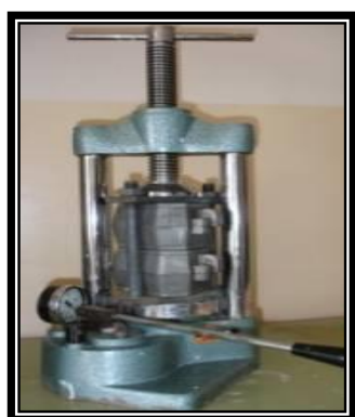
Figure 7: The flasks were placed under the two plates of the tension system while they were still placed under the hydraulic press.
