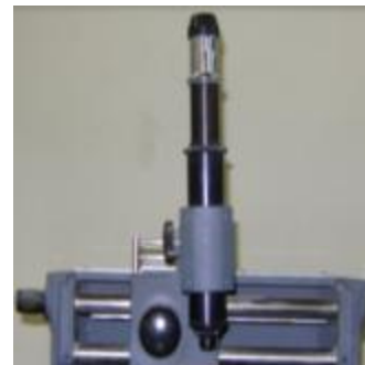
Figure 6: the optical travelling microscope which was used for measuring the vertical distances.
