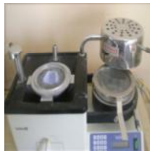
Figure 2: The stone cast with the thermoplastic record base attached to the biostar machine.
