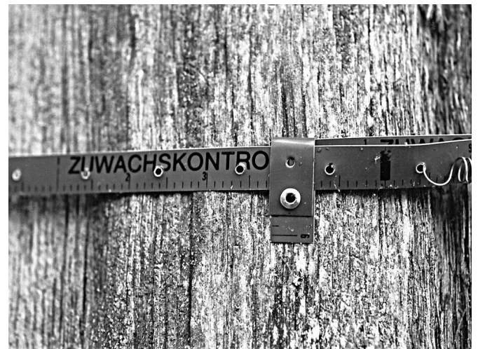
Fig. 13: Permanent measuring tape to record the change in the diameter of the Bear-Oak
