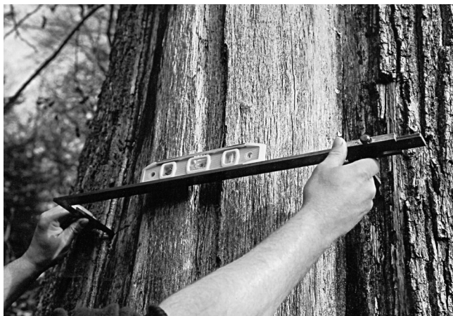
Fig. 11: Horizontally adjusted calipers for measuring the distance between both bulges
