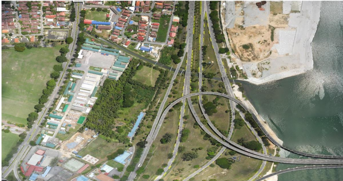
Fig. 5. Uncontrolled image mosaic of the selected area in Penang Island created with AutoPano Pro and PTGui software from 65 images taken by CropCam UAV on June 20th, 2011 (First Flight)
