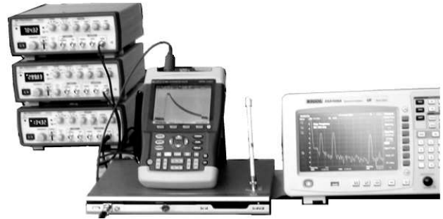
Fig. 9. A photo of the "LEMP Generator-Simulator" in a performance test
