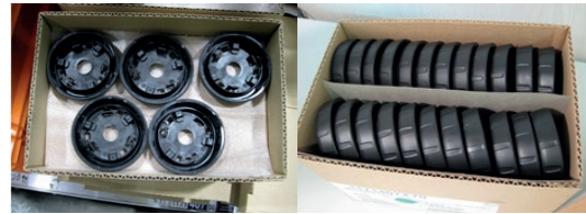
Figure 5. Improvement in placement of small component inside the box. Initial situation (left) and improved situation (right) (source: authors).
