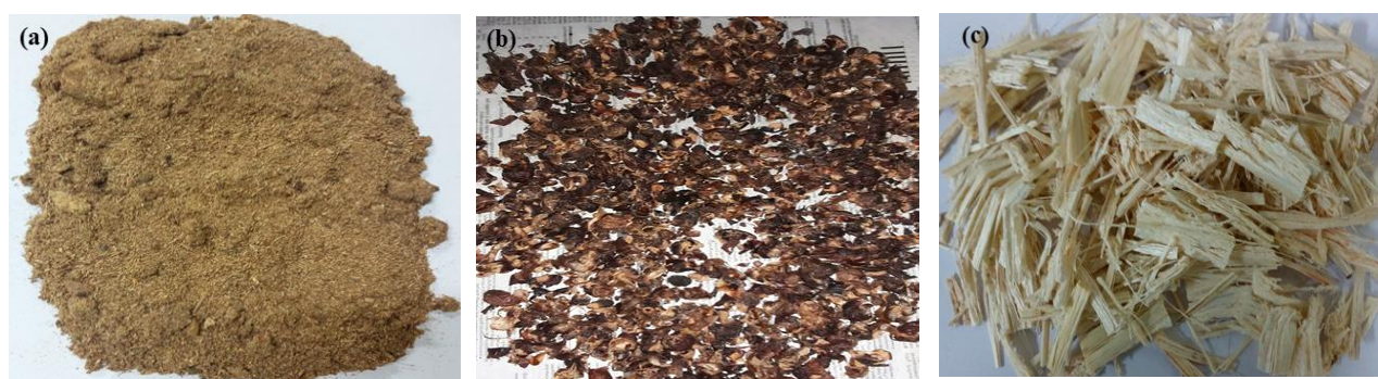
Figure No.1 Different Ligno-cellulosic biomass collected for biochar production, (a) Sawdust (SD), (b) Soapnut Pith (SP), (c) Sugarcane Bagasse (SB).
