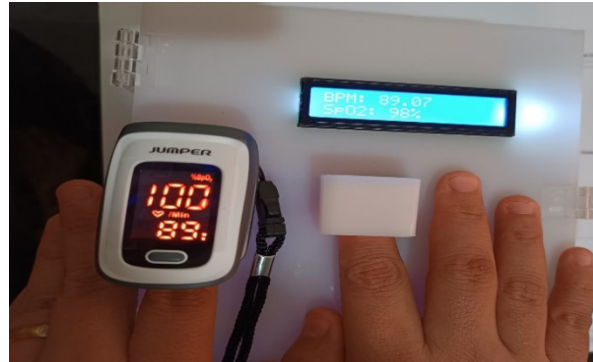
Fig. 7. Comparison of IoT-based pulse oximetry with Jumper brand pulse oximetry
