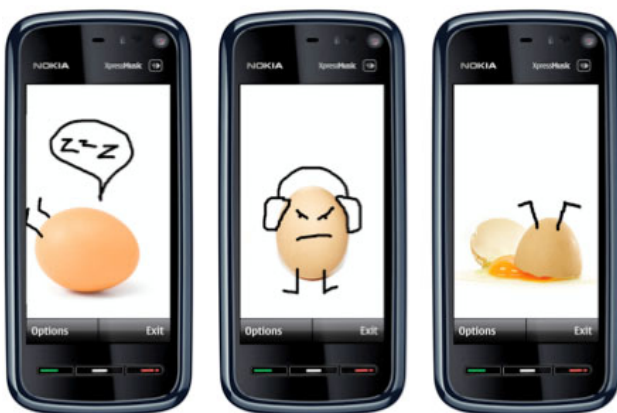
Figure 3. Three views of the prototype mobile application (from left to right): 1) measured sound pressure level is tolerable, 2) the sound pressure level is not appropriate and 3) the sound pressure level has exceeded the tolerable zone
