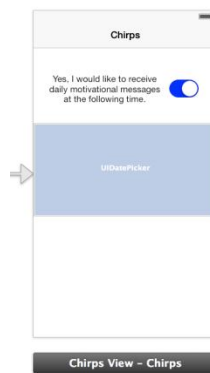
Fig. a12: Creating a new chirp’s view with a UIDatePicker and a UISwitch.
