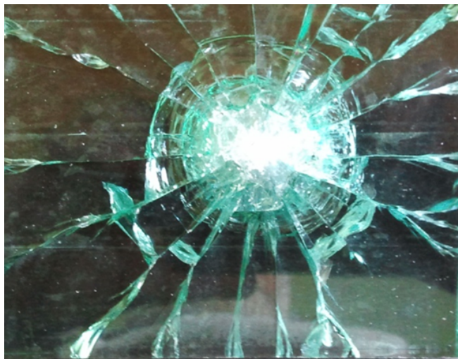
Fig.1: Glass plate after steel projectile impact at 74 \text{ ms}^{-1} showing comminuted cone at the center followed by circumferential cracks around the cone and large radial cracks. Occasionally a link up crack is also visible linking two radial cracks.
