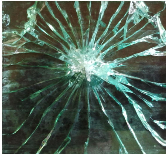
Fig. 3: Glass sample subjected to copper projectile impact at 66 \text{ms}^{-1} . Number of radial cracks are much higher than in the event of steel projectile impact.
