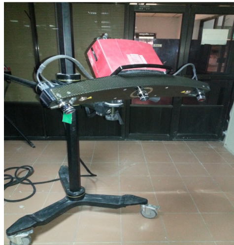
Fig. 5: ATOS Laser scanner setup.
