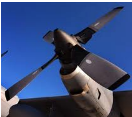
Fig. 2: Allison T56 turboprop engine with 4 propeller blades installed on C-130 aircraft.
