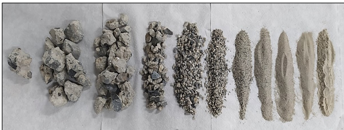
Fig. 3: Particle size distribution of one of the RCA samples evaluated.
