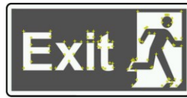
Fig. 9: The marker's features after extraction.
