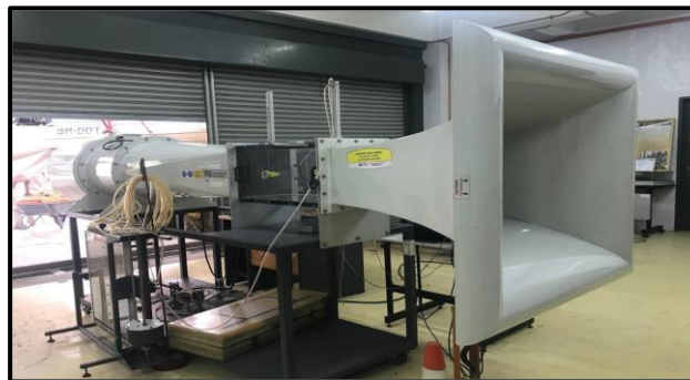
Fig. 1: The overview of AF100 Subsonic Wind Tunnel.
