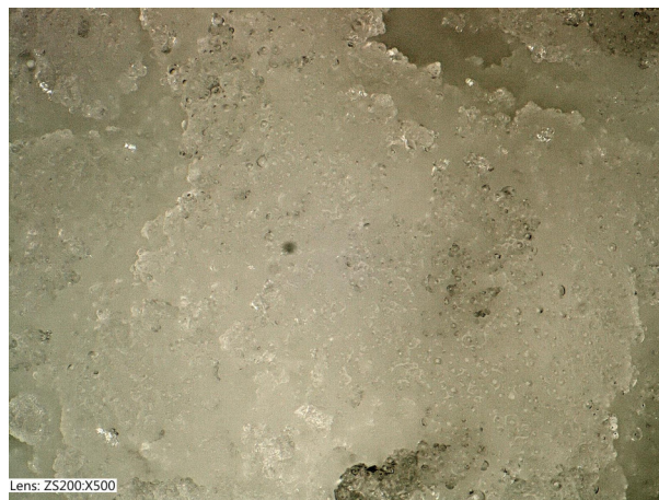
Figure 5. Image of microencapsulated sunflower-seed oil powder produced by a laboratory blender at 500× magnification.
