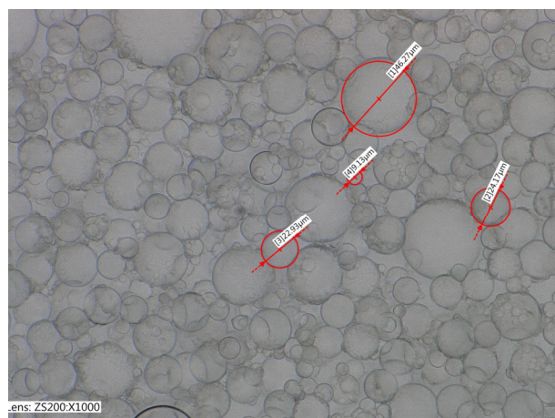
Figure 2. Microscopic image of emulsion sample at 1000 \times magnification.
