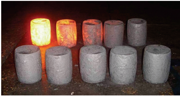
Figure 7 : Forgings made in experimental upsetting
