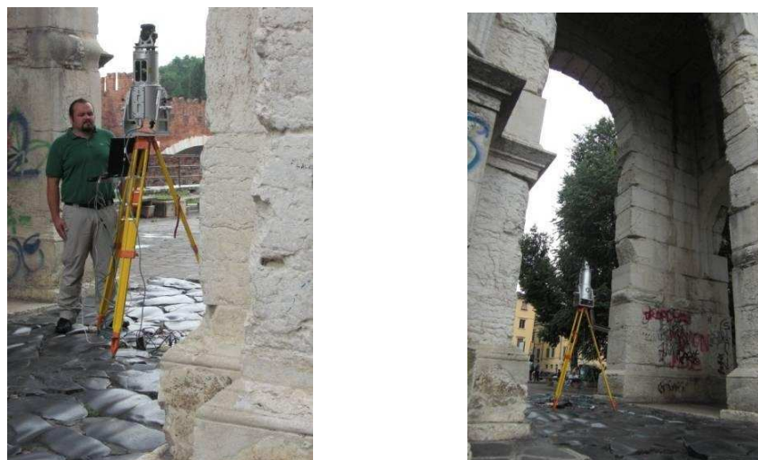
Figure 8;9. Recording with laser scanner of the inner and covered area of the arch
