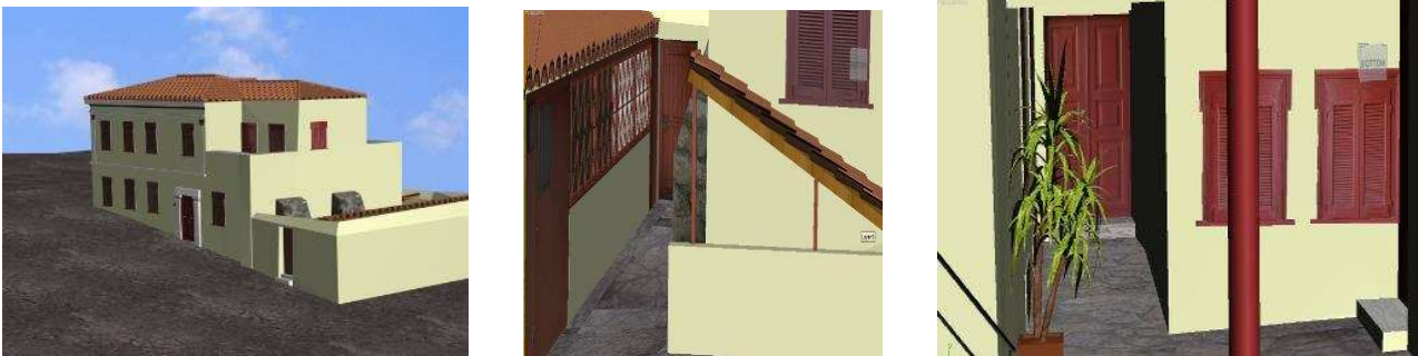
Figure 5: Perspective views of a 3D model building represented at the fourth LOD, in 3D Studio Max
