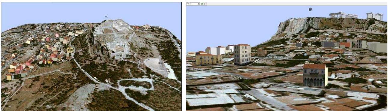
Figure 2: Left: Creation of the 3D background which resulted from a draping process. Right: Representation of buildings at the first level of detail (LoD).
