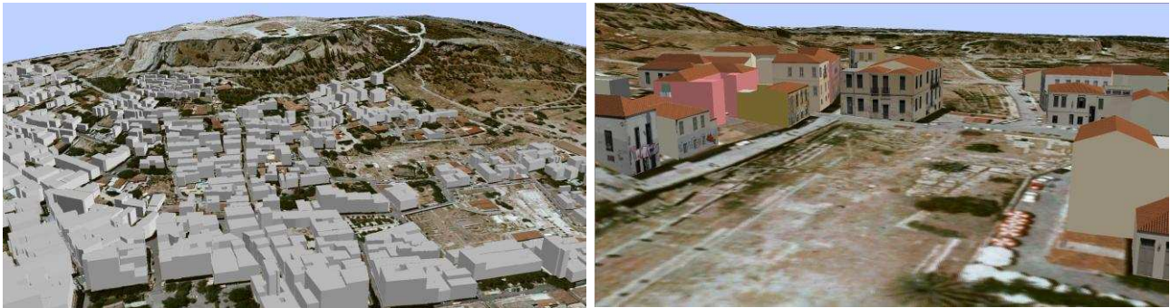
Figure 3: 3D representation of buildings at the second LoD (left) and at the third LoD (right) in ArcScene.
