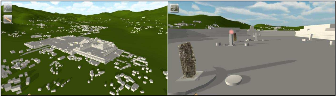
Figure 6: Navigation modes in QueryArch3D: [left] aerial view with LoD1 models only, [right] walkthrough mode, with mixed LoD1-to-LoD3 models. An example of the detail view for LoD4 models is given in Figure 2 (bottom-right).
