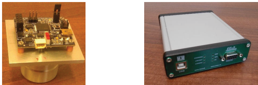
Figure 3: Tested devices: iNEMO STEVAL V2 MKI062V2 (left) and IMU EEaS (right)
