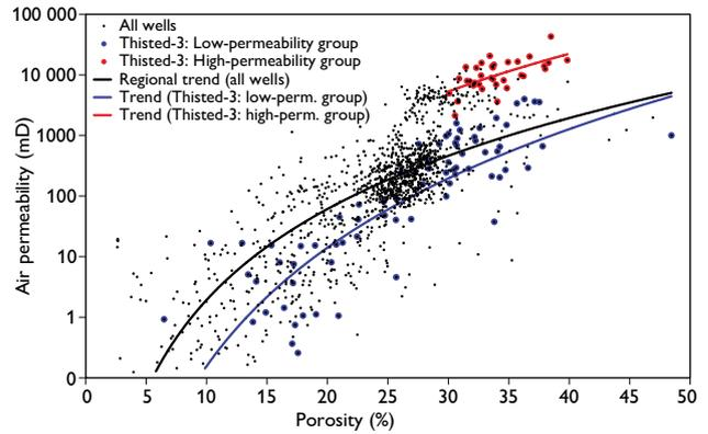
Fig. 4. Porosity–permeability plot based on conventional core analysis data from the Gassum Formation.
