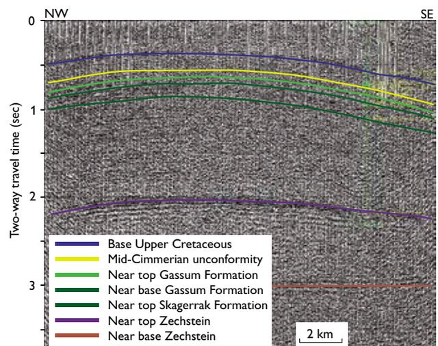
Fig. 2. Seismic section (PRKL7374A no 74249) across the Thisted salt pillow.
