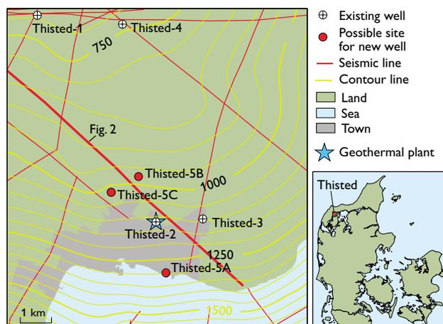
Fig. 1. Depth structure map of near top Gassum Formation (contour interval: 50 m) of the Thisted area showing seismic lines, well locations and possible locations of the planned Thisted-5 wells.
