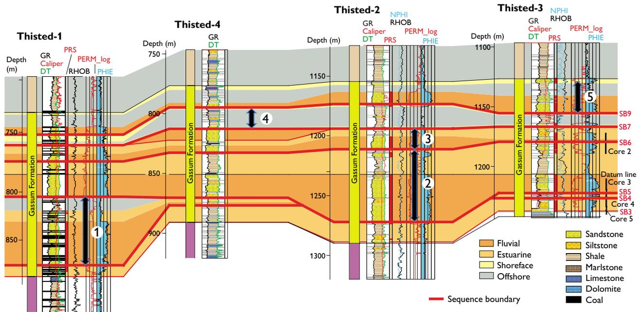
Fig. 5. Log correlation of sedimentary units within the Gassum Formation in the four Thisted wells. 1–5: sequences, red lines: sequence boundaries (corresponding to incised valley floors), PRS: potential reservoir sand. The sediments of the incised valleys are fluvial and estuarine.
