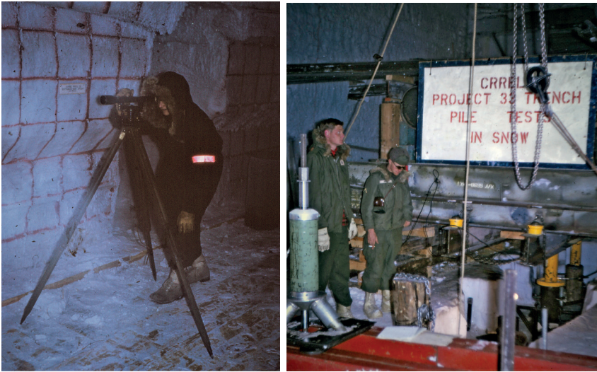
Fig. 2. USACE-applied glaciology research at Camp Century. Left: Measuring the deformation of firn in 1961. Right: Measuring the compressive strength of firn in 1964. Photos: Søren Gregersen.
