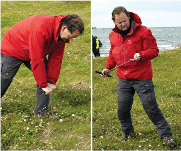
Fig. 2. Traditional geological mapping using the spear auger.
