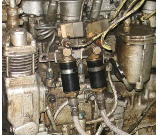
Fig. 2 Fuel system of the D-240 engine with solenoid valves to turn off the fuel supply of two ICE cylinders
