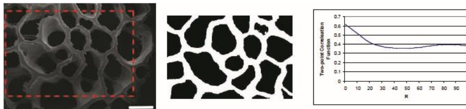
Fig. 12 Scanning electron photomicrograph of transverse slab of vertebral trabecular bone (left). The sample image after thresholding (middle). 2-point correlation function of pore (R represents the distance of two randomly selected points) (right). [26]
