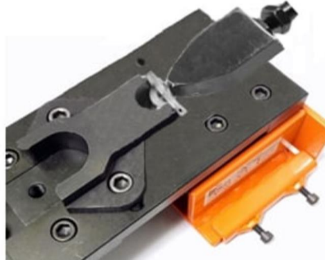
Fig. 1 Microbending machine, close-up of fracture toughness stage and sample
