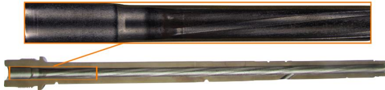
Fig. 7 Longitudinal section of the standard barrel
