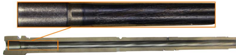
Fig. 8 Longitudinal section of the tested barrel
