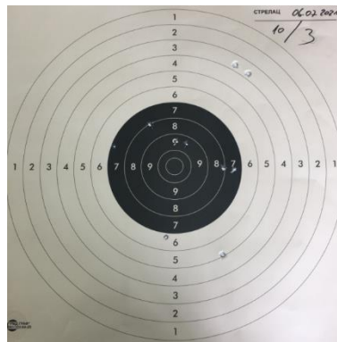
Fig. 1 One of the three targets after shooting 10 shots at 17000 rounds
