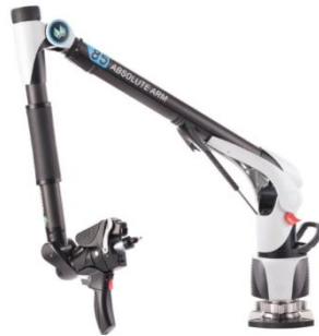
Fig. 9 3D scanner Hexagon RS5 with a stabilized Absolute arm platform 8525-7
