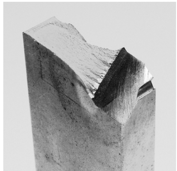
Figure 4. Fracture surface of DTD 5050 5½% Zn aluminium angle notch fracture toughness test specimen, initial \beta = 45^\circ .
