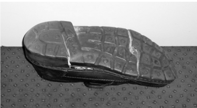
Figure 18. Cracks in sole of walking shoe.
