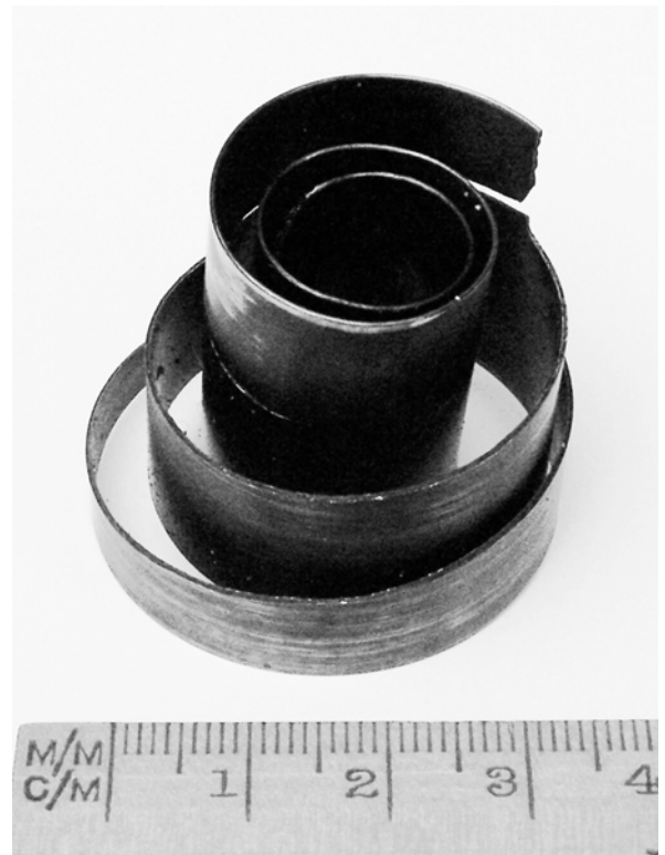
Figure 11. Centre portion of failed wall clock mainspring.
