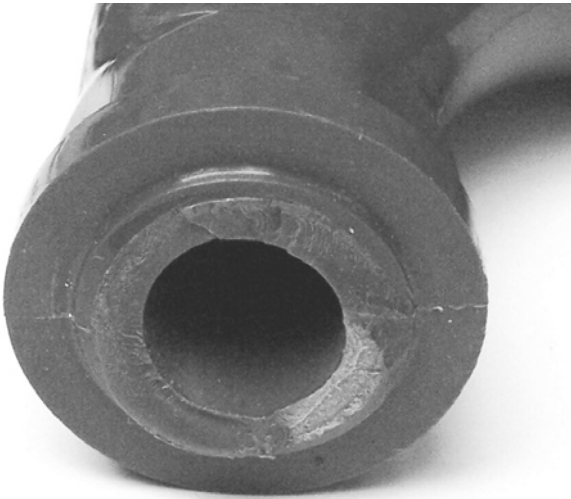
Figure 8. Crack surface of plastic domestic tap.
