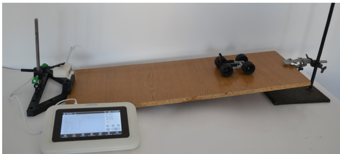
Figure 3: Experimental setup to study the characteristics of body motion on an inclined plane.
