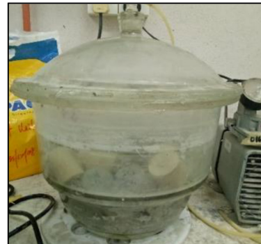
Fig. 2. Porosity test was carried out with the vacuum saturation method.
