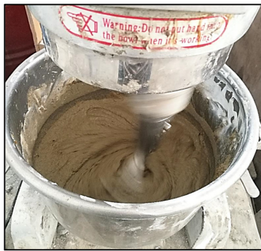
Fig. 1. A mortar mixer was used to prepare the lime mortar.
