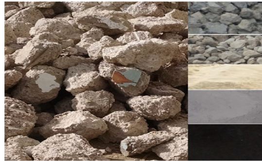
Fig. 1. Concrete ingredients: Large blocks of old concrete, recycled coarse aggregates after sizing, fine aggregates, and fly ash
